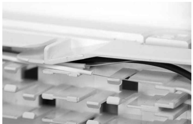
6.2 Recommended to strip the 900 micron to 250 micron half way the splice holder, in case of semi-tight pigtails. In case the pigtail is tight, only 0.8 m can be stored in the storage area.
